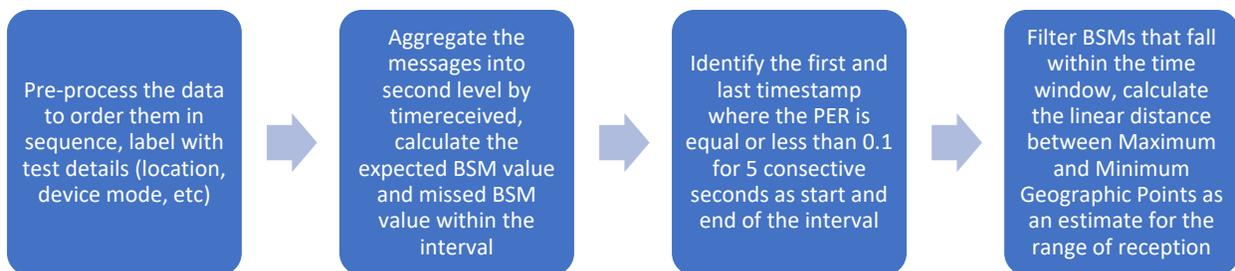
*Figure B1 Analysis Process Steps for PER Calculation*
