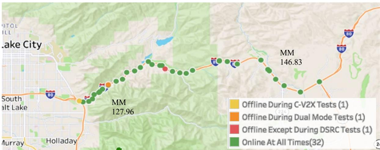
Figure 6 I-80 Test Location East of Salt Lake City (Note: Points show the 35 RSU locations on I-80)
