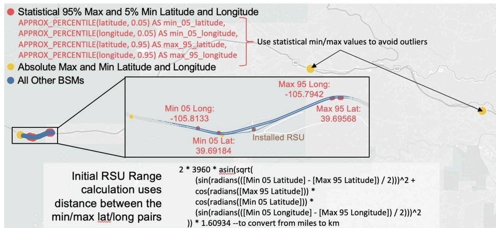
Figure C1 95/05 Percentile Range of Reception Calculation Concept and Calculation
