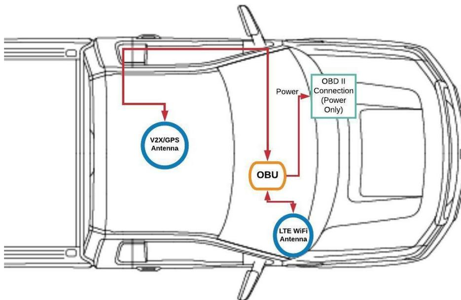
Figure 4 OBU Installation Diagram
