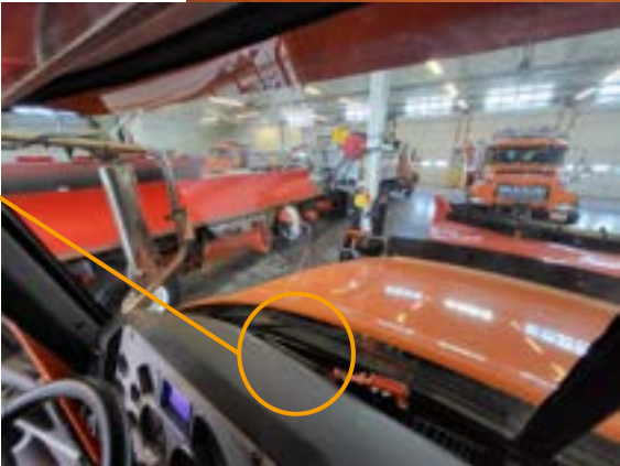
LTE antenna mounted on dash
